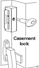
Fit locks which secure the frames together in preference to locks which simply secure the handle or stay bar. Casement windows, by their very design, need to be locked by securing the window to the frame. Most casement locks are screwed to the window rather than the frame - a weaker system. There are locks which are fixed to the frame and these are probably more secure, as well as being easy to use.
